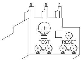
Figure 14. Over Current Relay
